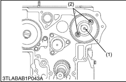
1. Camshaft                      2. Camshaft retaining bolt
