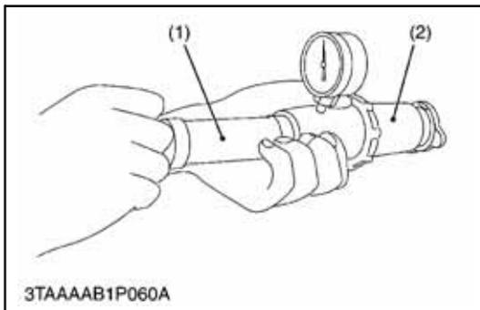
1. Attach the radiator cap to a pressure tester.
