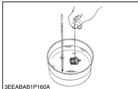
1. Suspend the thermostat in water by a string with one end of the string inserted between the valve and its seat.
