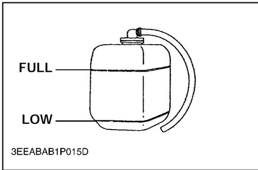
2. If the coolant level is too low, check the reason for the lost coolant.
