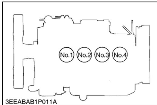
The cylinder numbers of V2203-DI (26-00119) series engine are designated as shown above. The sequence of cylinder numbers is given as No.1, No. 2, No. 3, and No. 4 starting from the gear case end of the engine.
